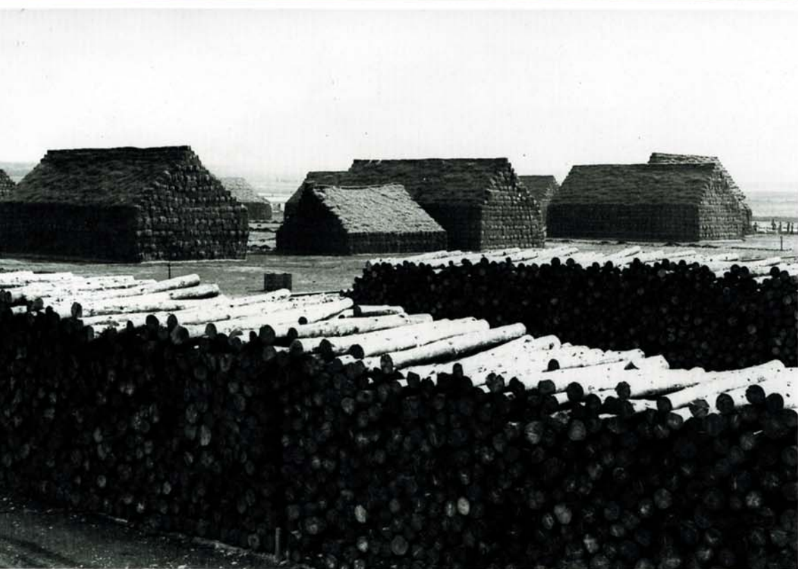
Stacks of straw and a pile of hardwood in the mill's storage yard, awaiting pulping.
