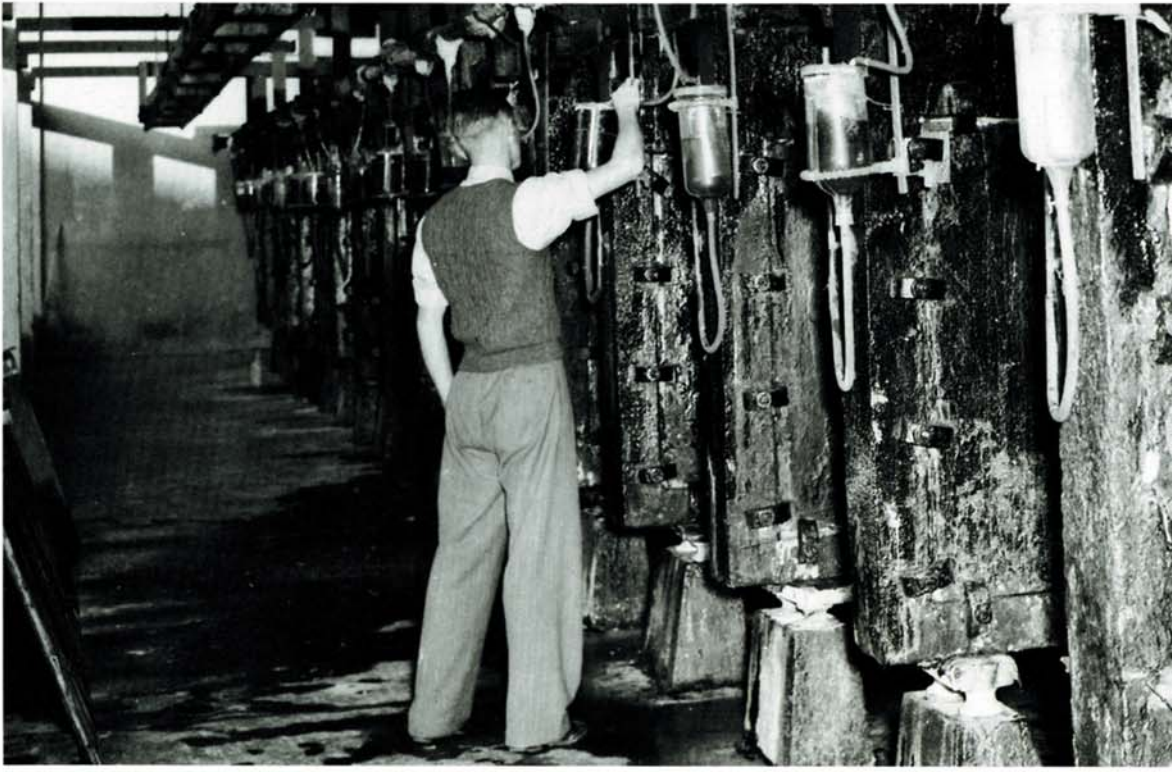
Electrolytic cells designed by Umberto Pomilio and capable of producing chlorine gas, caustic soda and hydrogen from salt.
