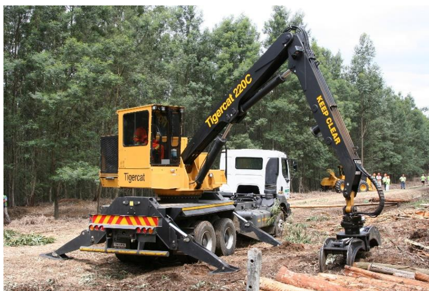
Photo 7: Truck-mounted knuckle boom loader. 6
