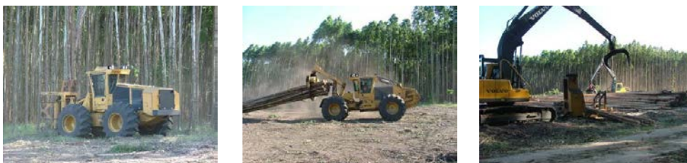
Photo 12: Equipment used in a multi-stem harvesting system (feller-buncher, grapple skidder, slasher deck).
