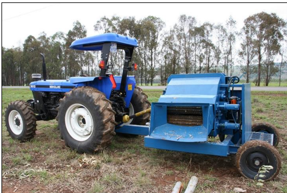
Photo 10: Locally manufactured small flail debarker
