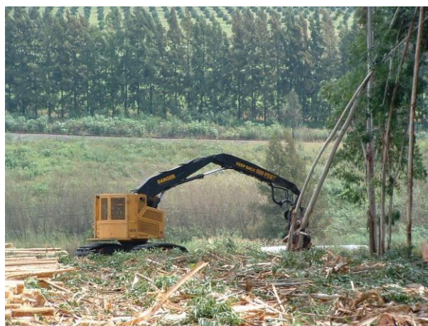
Photo 11a: Tracked single stem harvester (CTL system)
