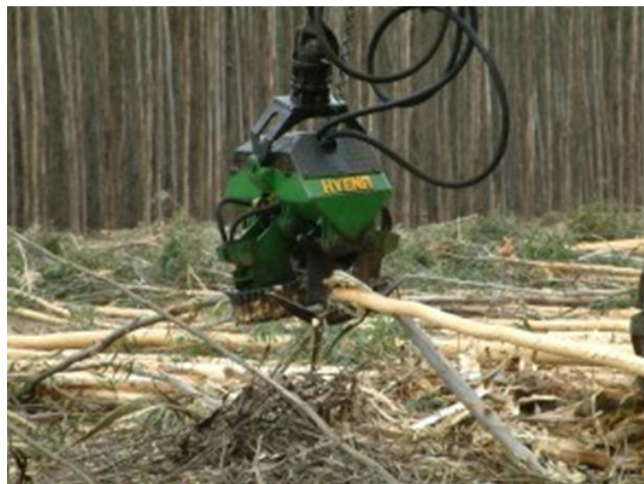
Photo 9: Locally designed debarking head 3
