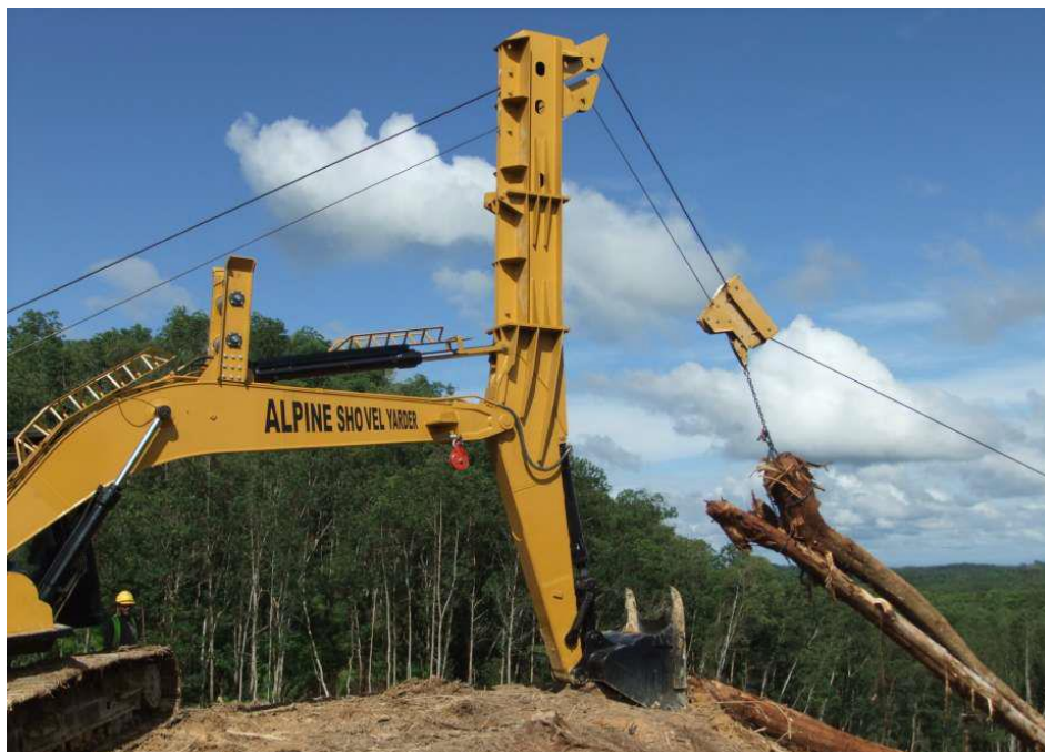
Photo 5: High power double drum shovel yarder with extended tower. 9
