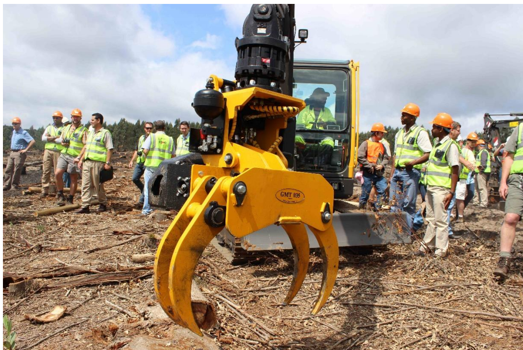
Photo 15: This felling grapple weighs just 225 kg and can be mounted on a truck-mounted crane, a three-wheeler, or a small excavator. It can cut standing trees up to 350 mm diameter. 8
