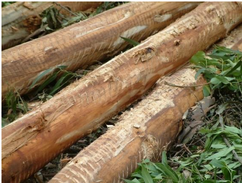
Photo 17 (left): Mechanically debarked timber 3
