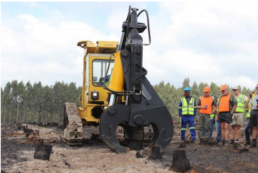
Photo 4: This de-stumper extracts stumps up to 600mm diameter by cutting them off 80mm below ground level. 2
