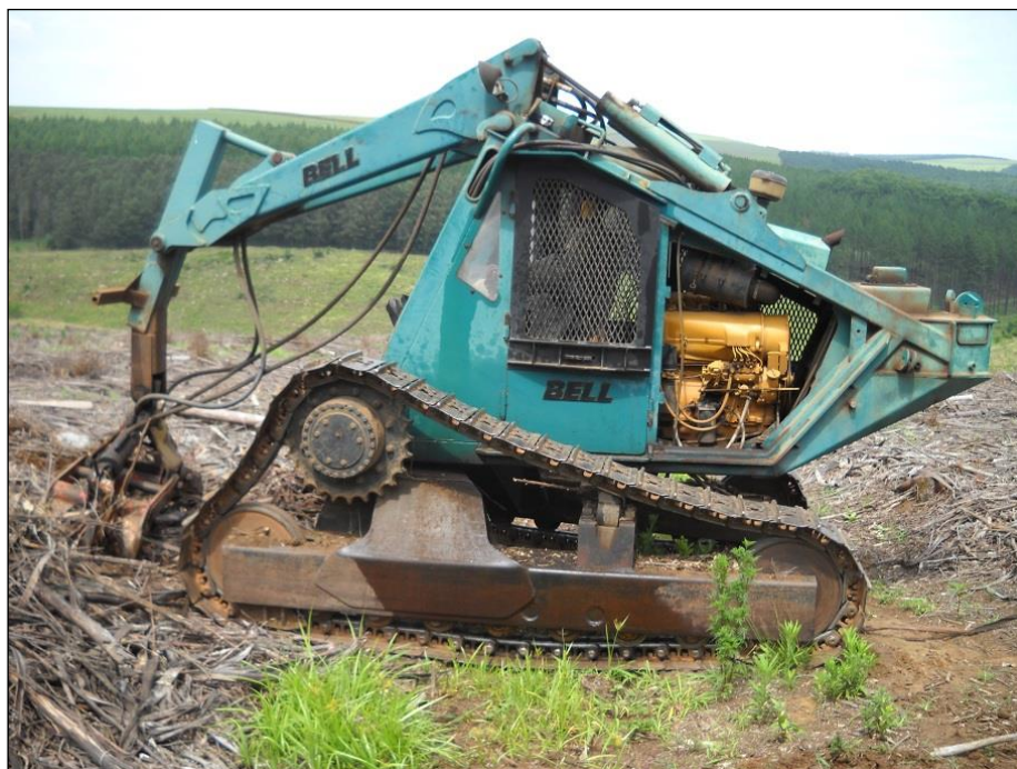
Photo 2: Logger converted as a pitter by Holley Brothers, Wartburg. 4
