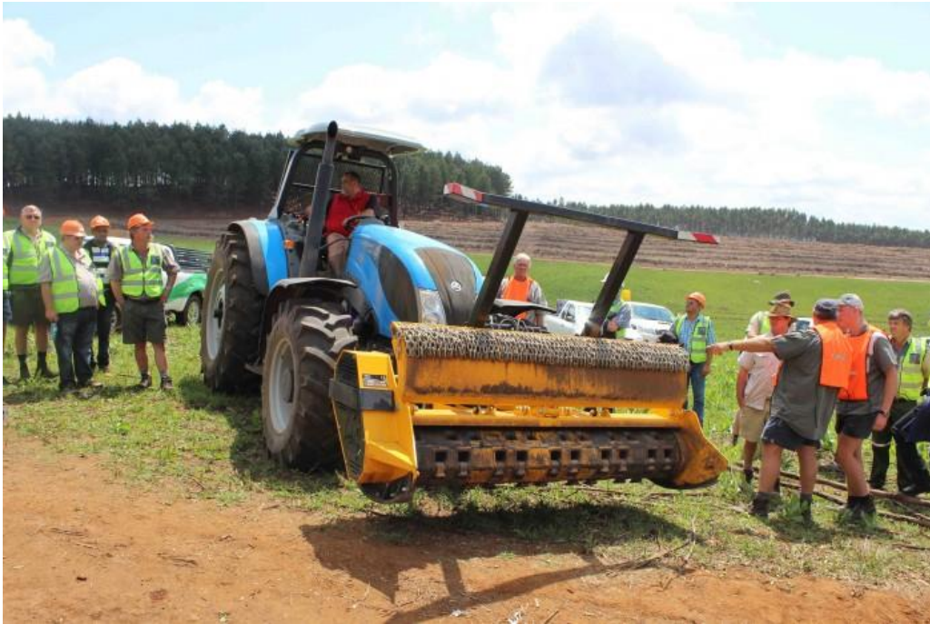
Photo 3: Lightweight mulcher ideal for the small-scale timber farmer. It needs a 100 Kw tractor. 2
