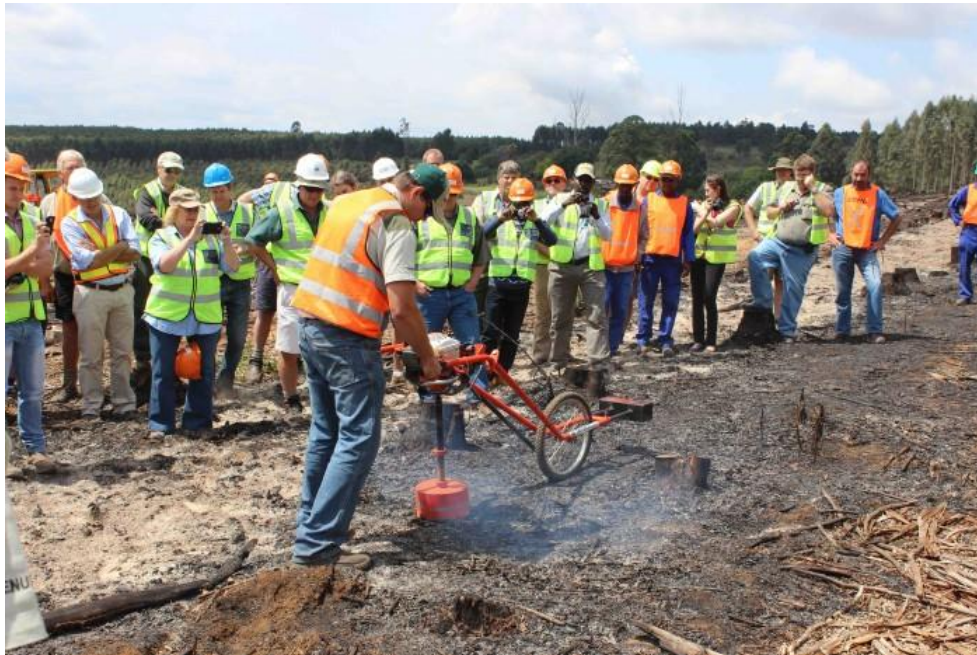
Photo 1: This innovative device is designed to take the weight of a mechanical pitter off the shoulders of the operator. 6
