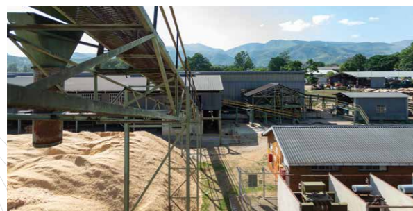
Sawdust, a renewable fuel, is used for the boilers (no fossil fuel is used).
